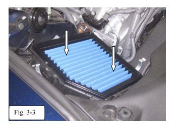
(c) Install the F-Sport filter into the lower air box housing (Fig 3-3).
