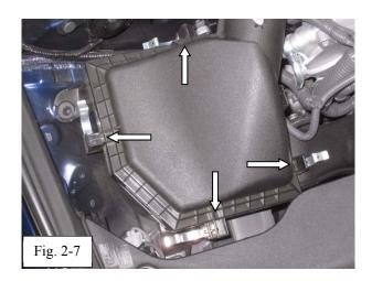
(g) Unclip the four (4) retaining clips on the air box lid and remove the complete assembly (Fig. 2-7).
