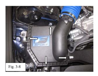
(i) Install the F-Sport air box lid into the bellows and engage the four (4) clips to secure the F-Sport air box lid (Fig 3-8).
