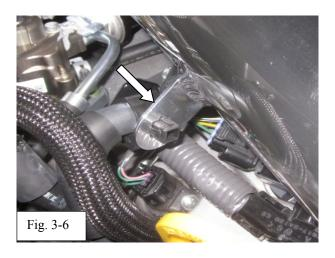
(f) Insert the hose clip into the retaining bracket on the F-Sport intake tube, making sure it is fully seated and snaps into place (Fig. 3-6).
