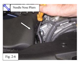
(f) Use needle nose pliers to unclip the wiring harness from the side of the factory air box lid (Fig. 2-6).
