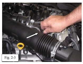
(c) Squeeze the clamp on the PCV hose, slide it back and disconnect the hose from the inlet tube (Fig. 2-3).
