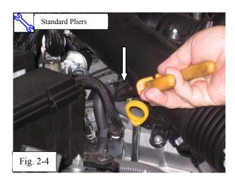
(d) Use standard pliers to unclip the hose from the retainer on the side of the inlet tube (Fig. 2-4).
