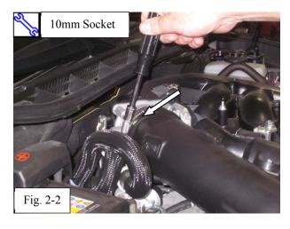
(b) Loosen the inlet tube hose clamp at the throttle body (Fig. 2-2).
