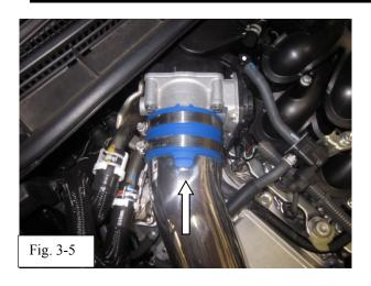
(e) Insert the F-Sport Intake Tube into the Coupler. **Do not tighten the hose clamp at this time** (Fig. 3-5).
