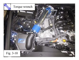
(k) Tighten the coupler and bellows hose clamps at the throttle body and air box (Fig 3-10).
