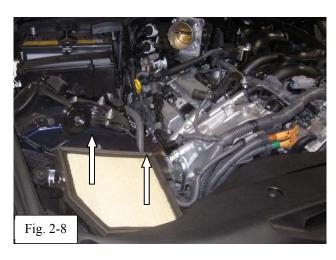
(h) Lift up to remove the factory air filter (Fig. 2-8).
