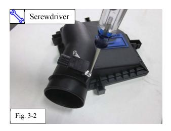
(b) Install the MAF sensor on the F-Sport Air Box Lid (Fig. 3-2).
