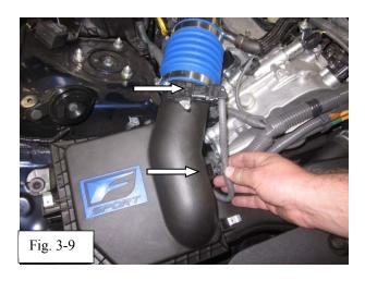
(j) Reconnect the MAF sensor and secure the wire clip to the side of the F-Sport air box (Fig. 3-9).
